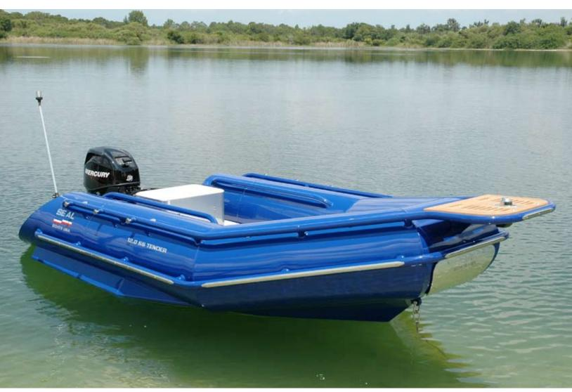
12.0 SS Tender with 25-HP Mercury, 4-stroke outboard motor.
