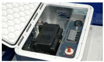
Built-in battery in seat box with on/off switch, fuel gauge and electrical switches.
